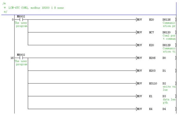
Above demo means plc com2 is Modbus master, communication parameter is 115200, 1, 8, even.
