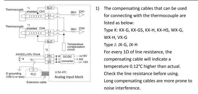
Therefore a short (less than 100m) compensating cable is recommended. Unused channels should have a wire link connected between the + and – terminals to prevent an errors being detected on that channel.
