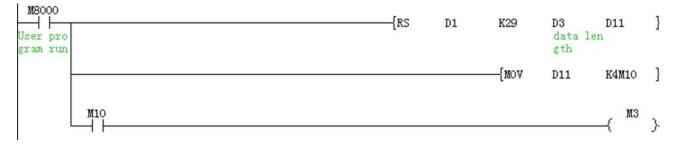
BFM29 (K4M10) assign value to m25<sup>~</sup>m10. When there is an error, m10=1. M10 is the bit0 of BFM 29.
