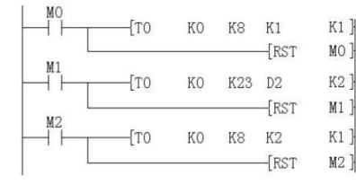
Step 1: Remove all weights; Step 2: Write 0x0001 to #8; Step 3: Add known weights; Step 4: Write known weights (D2) to #23; Step 5: Write 0x0002 to #8
