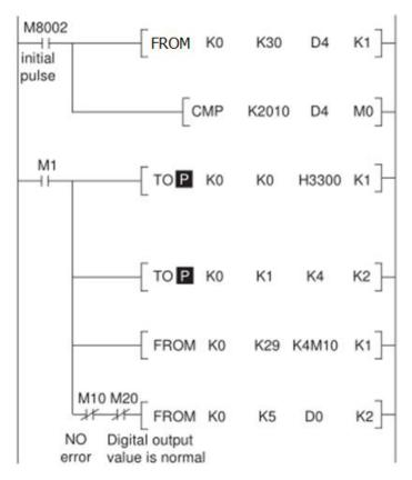
The FROM code for the special function block at position "0" is read from BFM #30 of that block and stored at D4 in the main unit. CMP is compared to check the block is a LX3V-4AD, if OK M1 is turned ON. These two program steps are not strictly needed to perform an analog read. They are however a useful check and are recommended as good practice.
