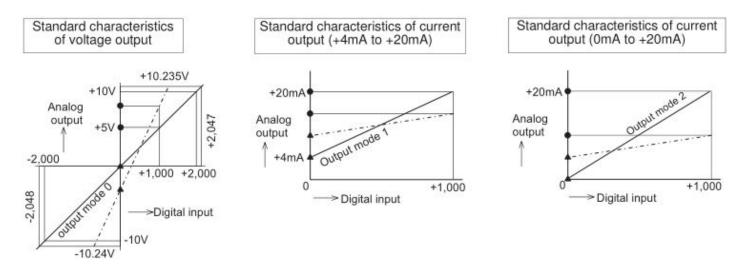
• . . . Gain value : Analog output value when the digital input is +1,000
