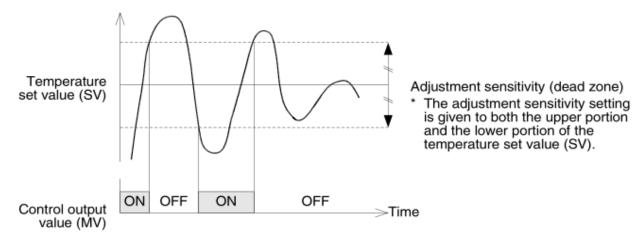
When the dead zone sets to a large value, vertical fluctuation would be larger. But if dead zone is too small, small oscillations of the measured value may cause vibration.
