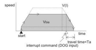
• Two-speed positioning operation
