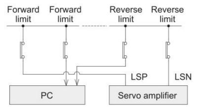
Because a drive amplifier for a stepper motor does not have these terminals, make sure to provide limit switches on the PLC. Evade from the state of the pulse output stop by Jog in the opposite direction when forward pulse stop or reverse pulse stop is turned on.
