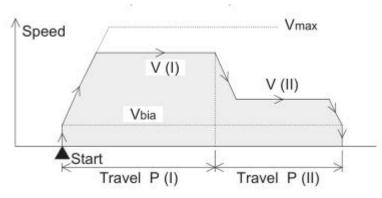
The motor performs the following operation by the two-speed positioning operation command. Approach at high speed as well as processing and moving forward at low speed can be performed. When the start command is received, the motor performs positioning at the operating speed V(I) (BFMs #20 and #19) until the set position P(I) (BFMs #18 and #17), then at the operating speed V(II) (BFMs #24 and #23) until the set position P(II) (BFMs #22 and #21) (two-step speed).
