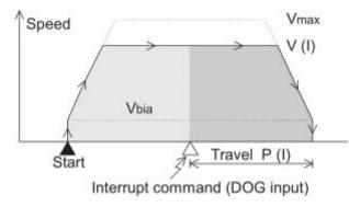
When the start command is received, the motor starts operation. When the INTERRUPT input is received, the motor moves by the specified distance, then stops (The relative travel exclusively can be specified.) The current value is cleared by the start command. The current value starts to change by the INTERRUPT input, and becomes equivalent to the set position when the operation is completed.
