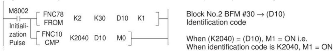
This initial step checks that the special function block placed at position 2 is actually an LX2N-4AD-PT, i.e. its unit identification number is 2040 (BFM #30).
