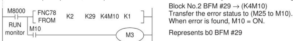
This step provides optional monitoring of the LX2N-4AD-PT Error Buffer Memory (#29). If there is an Error on the LX2N-4AD-PT, bit b0 of BFM #29 will be set on.
