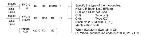
This initial step checks that the special function block placed at position 2 is actually an LX3V-4TC, i.e. its unit identification number is 2030 (BFM #30). This step is optional, but it provides a software check that the system has been configured Correctly.
